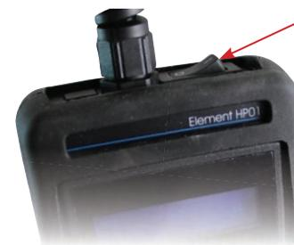
Operate the breaker on the controller (disconnect the power plug).
