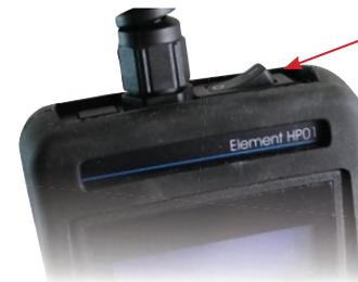
Operate the breaker of the controller (disconnect the power plug).
