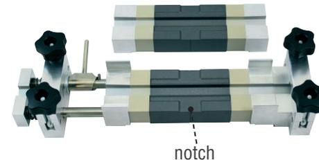
Apply the upper part of the mould accurately, then fit the lower part of the mould.
