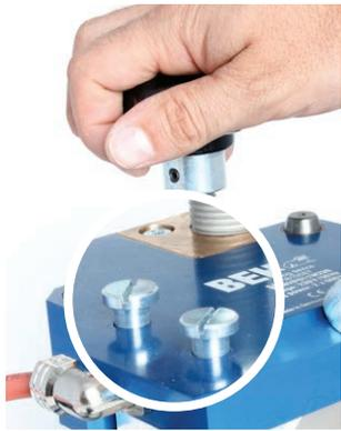
Turn the star handle to the right until the above and lower moulds are touching. Thereafter star handle continue to turn until the screw heads stand 3-4 mm from the upper case plate.
