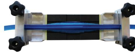
Leave the mould and profile within the closed machine until the temperature is cooled down. The current temperature of the heating plates is shown in the display of PPuls controller.
