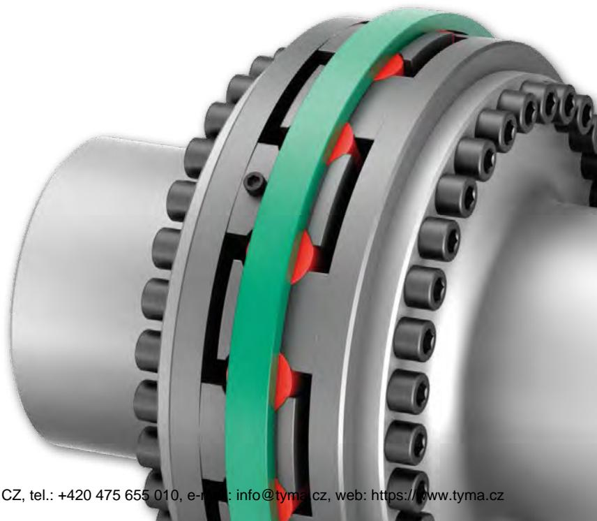
Replacement of elastic buffers without axial movement of the coupled machines. After removing the cheese head screws the retaining ring can axial shift and the buffers are free changeable each by each.
