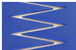
Finger joint with a hot press
