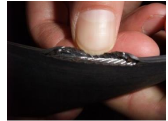
Fig. 33: Damaged traction member [ContiTech]
