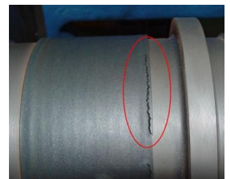
Fig. 35: Longitudinal crack on reverse [ContiTech]
