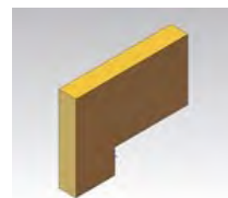
AN = Angular Shape: two portions of the cleat are set at an angle to each other
