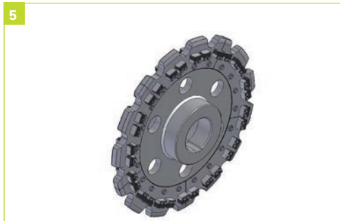
Figure 5 and 6: Sprocket with special rectangular noise dampers
