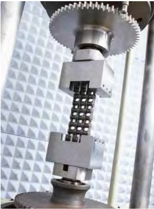
Fatigue strength determined with a high-frequency pulser
