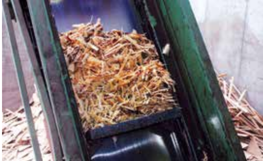
Wood chips conveyor at root reducer and trimming station
