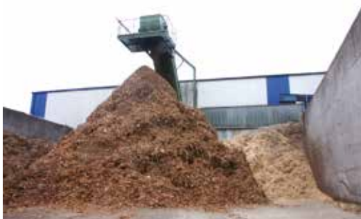
Wood chips conveyor at debarking station
