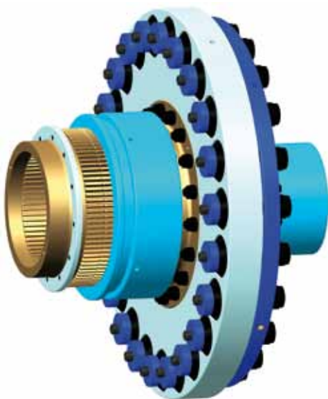
flexible pin type coupling shiftable at standstill, buffers prestressed and electrically insulating, bolts hydraulically demountable
